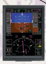
Four, DU-1080 LCD configuration: Full flight deck integration featuring two PFDs and MFDs. Offers increased redundancy and enhanced pilot situational awareness.
